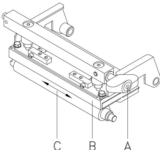
A soiled print roll can lead to reduced print quality and can affect transport of material.
