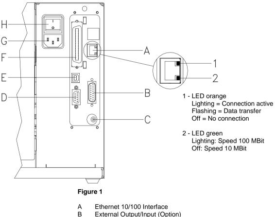
**Connector Pin Assignment (Printer Rear)** 1.4
