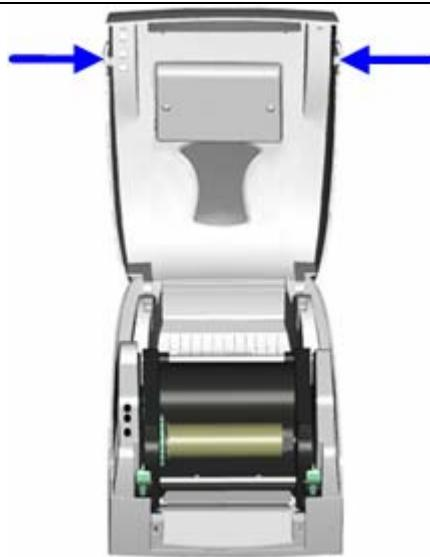
2. Loosen and then lift the upper print mechanism by pressing the locking tenons.
