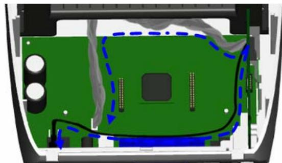
16. Thread Antenna Connection Wire through the hole on the Antenna Bracket. Then put the Antenna Connection Wire and Antenna Bracket on the Antenna port as figure showed.
