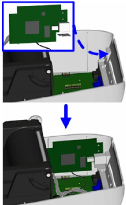
14. Secure the module onto the back plate.
