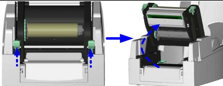
3. Place a new ribbon roll onto the ribbon supply shaft.
