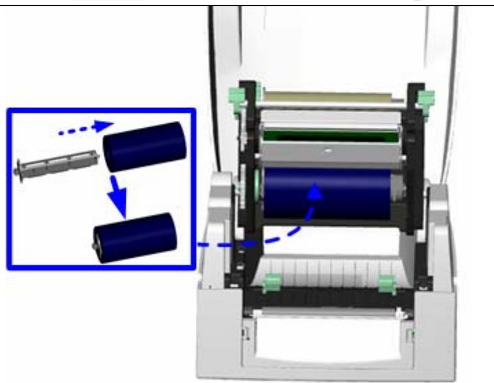
4. Feed the ribbon from the Ribbon Supply Shaft under the Print Head.
