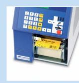
The dispending unit separates the label from the carrier and provides it for further processing. After removing the label, the following print order is activated by the dispenser photocell or an external impulse.
