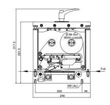
» Dynacode IP print mechanics right hand version, continuous mode
